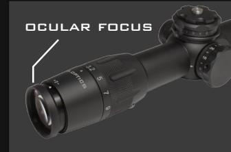
THE OCULAR FOCUS RING IS USED TO FOCUS THE RETICLE. DIOPTRER ADJUSTMENT IS FROM +2 TO -3. DO NOT USE THE EYEPIECE TO ADJUST THE SIGHT PICTURE OR TO ADJUST PARALLAX.
