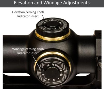
The TS-6X and TS-8X feature 1/4 MOA clicks on both the elevation and windage knobs. The elevation and windage knobs feature an indicator insert marked with directional arrows and reference points at 0, 4, 6, 8, 16, 8. Each hash mark = 1/4 MOA adjustments
