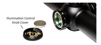
To install the battery, insert a CR2032 battery with the positive side (+) facing outward. To secure the battery in place, attach the illumination control knob cap by turning it clockwise.
