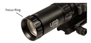
The focus ring is used to focus the reticle. Focus prescription ranges from +2 to -3. Do not use the focus ring to adjust the sight picture or to adjust for parallax.
