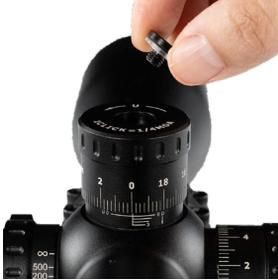
6. While holding the elevation knob in place, use a flathead screw driver to tighten the screw back on. Rotate clockwise until you feel resistance. Do not over tighten.
