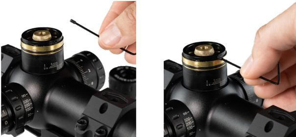
6. Screw the set screw clockwise until it sits flush with the elevation knob base.
