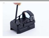
Use a flathead key to make elevation adjustments to your red dot's position. As indicated, counter-clockwise moves your Point of Impact down. 1 Click = 1 MOA
