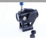
Use a flathead screwdriver to make elevation adjustments to your red dot's position. As indicated, counter-clockwise moves your Point of Impact up. 1 Click = 1 MOA
